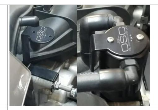
Use light oil on the fitting into rubber connector on intake manifold (near PCV cap)
